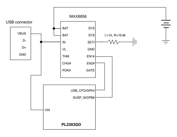
Figure 10-7b Battery Charging Design Example #2
