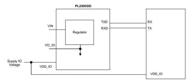
Figure 10-4b VDD IO Voltage Supply
