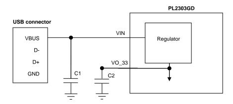
Figure 10-1 USB Bus Powered Design Example
