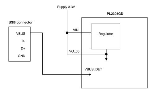
Figure 10-2b USB Self Powered Design Example 2
