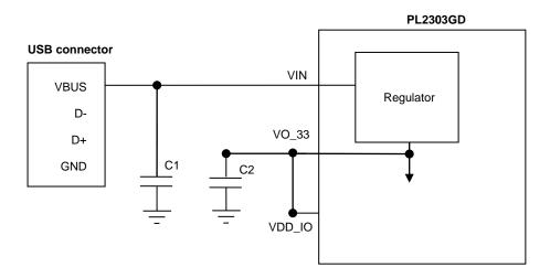
Figure 10-4a IO Power Supply
