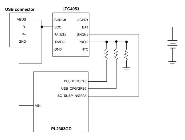
Figure 10-7a Battery Charging Design Example #1
