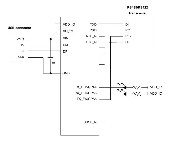
Figure 10-6 USB to RS485/422 Design Example
