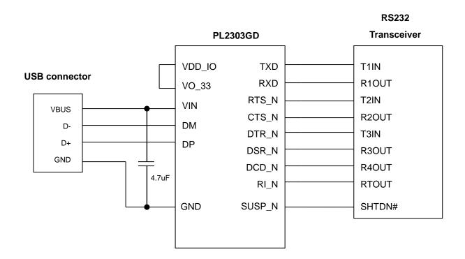
Figure 10-5 USB to RS232 Design Example
