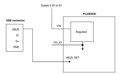
Figure 10-2a USB Self Powered Design Example 1
