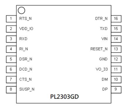
Figure 7-1 PL2303GD Pin Diagram (SSOP16)
