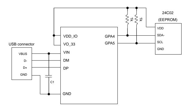
Figure 10-8 External I2C EEPROM Design Example
