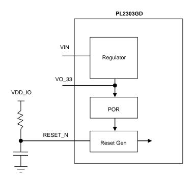
Figure 10-3a Chip Reset Control Application
