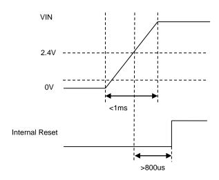
Figure 10-3b Chip Power Reset Timing Diagram
